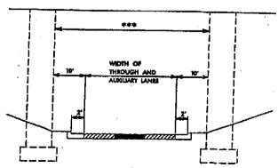
CURB AND GUTTER APPROACH WITH AUXILIARY LANES
